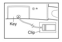
of your clothes. Then, insert the key into the console. After a moment, the displays will light. IMPORTANT: In an emergency situation, the key can be pulled from the console, causing the walking belt to slow to a stop. Test the clip by carefully taking a few steps backward; if the key is not pulled from the console, adjust the position of the clip.
